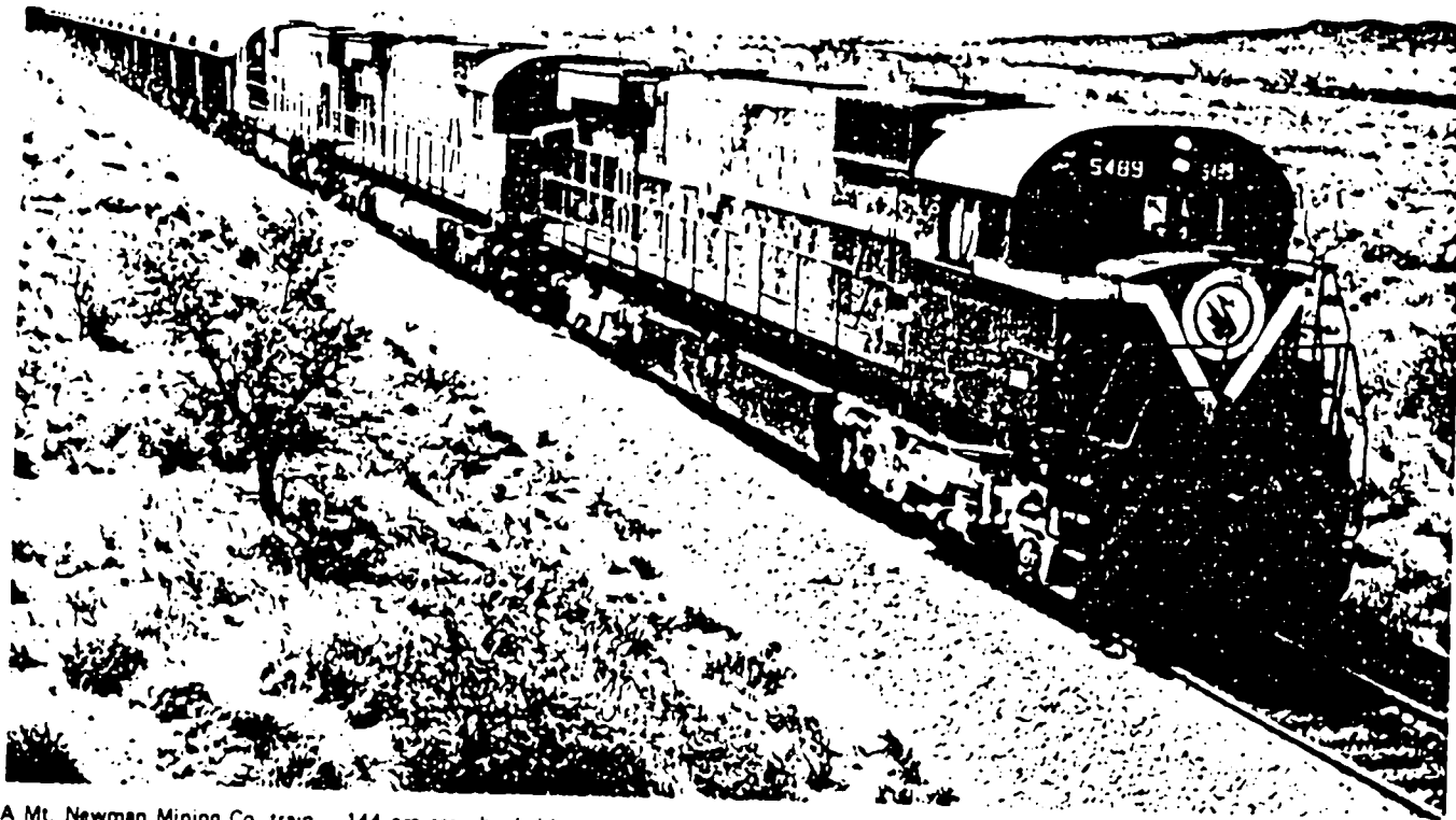
A Mt. Newman Mining Co. train - 144 ore cars, hauled by three locomotives, heads for the Mine at Newman after dumping its load 426km away, at Port Hedland. The round trip takes 19.5 hours, and there is a total of 69 trains a week every week of the year.
